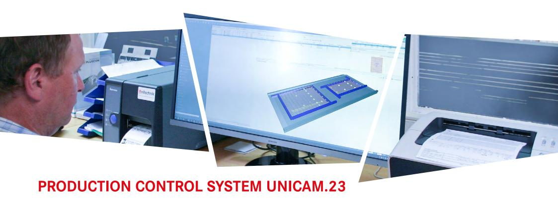
The UniCAM production control system is the heart of the precast concrete plant. The control system acts as a link between design and production as well as the precast component warehouse. Based on the individual CAD data, UniCAM plans and optimizes the production process.
