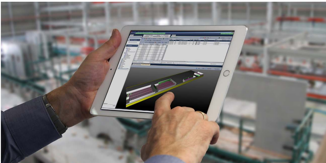
The production control computer (here UniCAM.10) receives a comprehensive picture of the products that are to be produced on the system. ©Unitechnik
