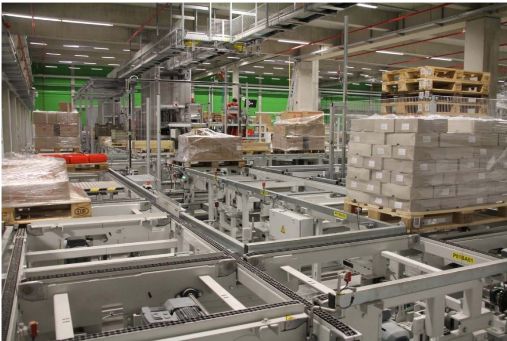
Providing for a capacity reserve is worthwhile when designing the conveyor system ©Unitechnik
